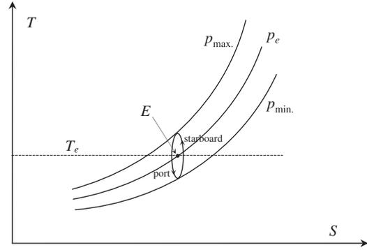
Fig. 2. Qualitative portrait on the temperature-entropy plane of the cyclic thermodynamic evolution of the air mass inside the tank chambers ( $E$ : equilibrium conditions). The cycle area is magnified for clarity reasons.
