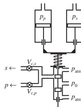
**Fig. 5.** Scheme of air pressure restoring device.
