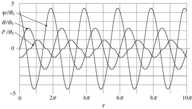
**Fig. 3.** Example of Euler–Cauchy numerical solutions for the case of non-linear efflux through valve  $V_c$ . Data:  $J_1=0.05$ ,  $J_2=0.0005$ ,  $\omega_w/\omega_s=1.4$ ,  $\omega/\omega_s=0.9$ ,  $K_p/J_1=5$ ,  $B=4$ ,  $d_\theta=0.15$ ,  $d_\psi=0.01$ ,  $C_f=5$ ,  $C_t/\sqrt{\theta_0}=27.426$  ( $C_{t, \text{equivalent}}=30$ ),  $C_{l, \text{laminar}}$  stability threshold=12.755.
