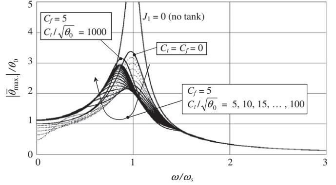
Fig. 6. Frequency response for various efflux coefficients  $C_t$ . Dots: unstable. Thick line: stable. Thin line: linear stability, non-linear instability. Data:  $J_1 = 0.05$ ,  $J_2 = 0.0005$ ,  $\omega_w/\omega_s = 1.4$ ,  $K_p/J_1 = 10$ ,  $B = 4$ ,  $d_\theta = 0.15$ ,  $d_\psi = 0.01$ .
