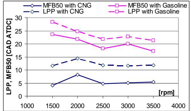
**Figure 3 MFB50 and LPP values for both gasoline ( $\lambda$  reported in Figure 1) and CNG ( $\lambda = 1$ ) operation at full load**
