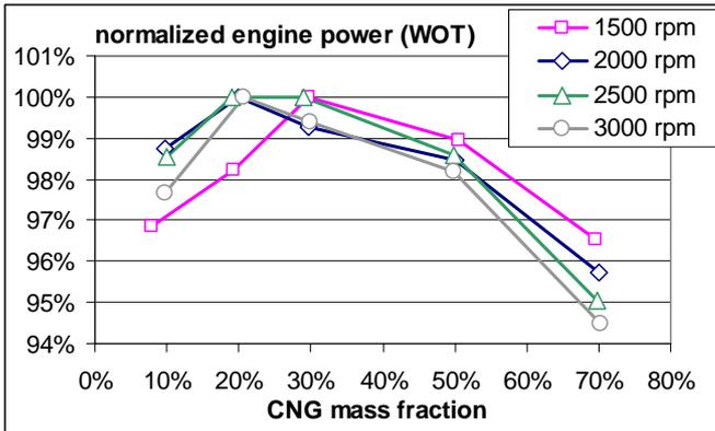
**Figure 8 Normalized engine power measured in double-fuel mode at WOT and  $\lambda=1$**
