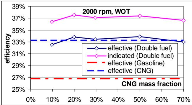
**Figure 5 Indicated and effective efficiency for Double-fuel (overall  $\lambda=1$ ), gasoline ( $\lambda=0.84$ ) and CNG ( $\lambda=1$ ) operation**
