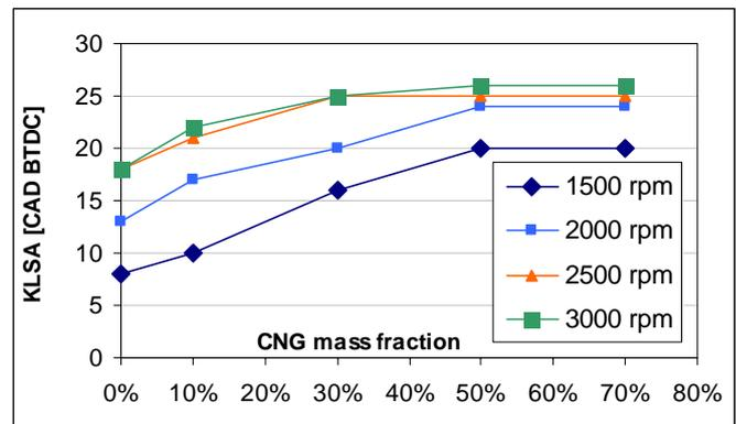
**Figure 4 Knock Limited Spark Advance measured at WOT both for pure gasoline (CNG=0%,  $\lambda$  reported in Figure 1) and double-fuel combustion (overall  $\lambda = 1$ )**
