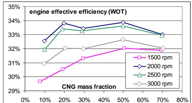
**Figure 7 Effective efficiency measured in double fuel-mode at WOT and  $\lambda=1$**
