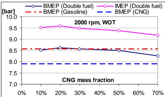
**Figure 6 IMEP and BMEP for Double-fuel (overall  $\lambda=1$ ), gasoline ( $\lambda=0.84$ ) and CNG ( $\lambda=1$ ) operation**
