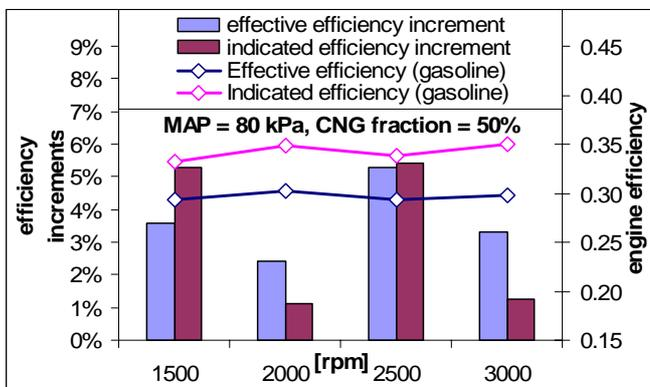
**Figure 12 Efficiency improvements obtained with respect to gasoline (MAP=80 kPa,  $\lambda=1$ , CNG mass fraction=50%)**
