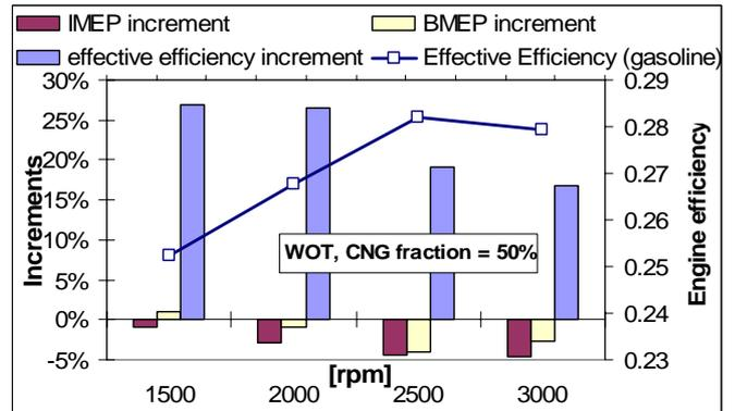
**Figure 9 Improvements obtained at WOT and  $\lambda=1$  with CNG mass fraction=50%**
