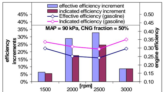
**Figure 11 Efficiency improvements obtained with respect to gasoline (MAP=90 kPa,  $\lambda=1$ , CNG mass fraction=50%)**
