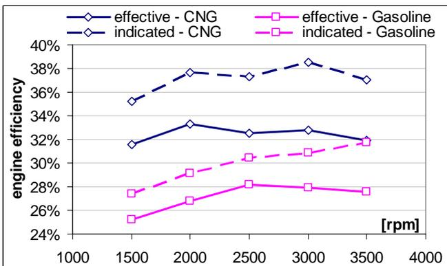
**Figure 2 Indicated and effective efficiency for both gasoline ( $\lambda$  reported in Figure 1) and CNG ( $\lambda = 1$ ) operation at full load**
