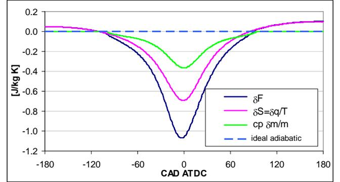
figure 4 Loss function variation  $\delta F$  and its constitutive terms vs. crank position ( $\delta \theta=1$  crank angle degree).
