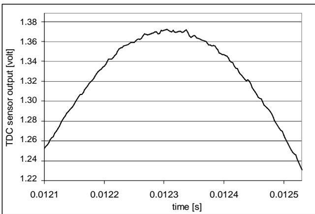
figure 6 A typical TDC sensor signal acquired with 0.005 ms resolution (1500 rpm)
