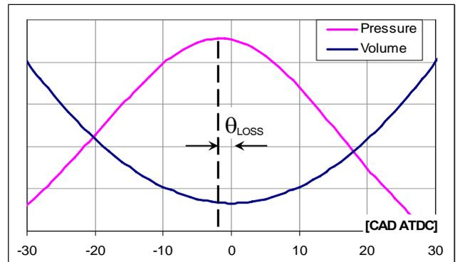
figure 2 Qualitative progress of in-cylinder pressure and volume near TDC
