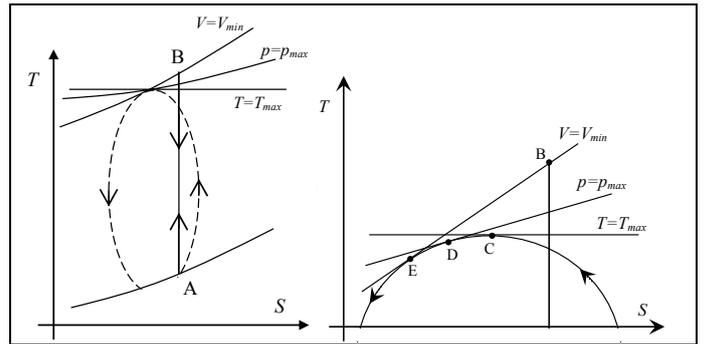
figure 1 Temperature-Entropy diagram of the compression-expansion process in a motored cylinder: ideal engine (segments AB and BA) and diabatic engine (dashed curve); the peak pressure (point D) occurs before the TDC (point E).
