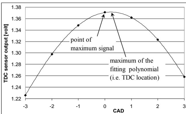
figure 7 An example of TDC sensor signal, acquired with 1 CAD resolution, fitted by a 4<sup>th</sup> degree polynomial
