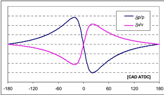
figure 3 Qualitative progress of  $\delta V/V$  and  $\delta p/p$  ( $\delta \theta=1$  crank angle degree)
