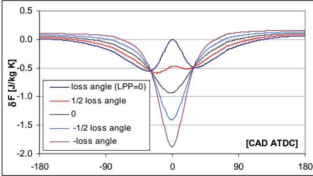
figure 5 Loss function increment  $\delta F$  for different phase errors ( $\delta\theta=1$  crank angle degree)
